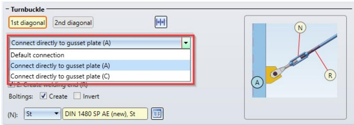
Previously, the turnbuckles' blade screws were connected to the gusset plates via a connecting plate. A selection list has been added to the **Fixing** tab, where you can choose to connect the blade screw to the gusset plate on one side of the two diagonals without a connecting plate, in addition to the **Default connection**. On the other side of the diagonal, the blade screw is still connected to the gusset plate via a connecting plate.
