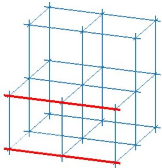
In the upper image, for example, the Y-axes labelled **1** are selected in the table and the lines in the graphic are marked red accordingly. Since the Y-axis **1** is hidden on the top plane, the X-axes in this plane are also shortened.
