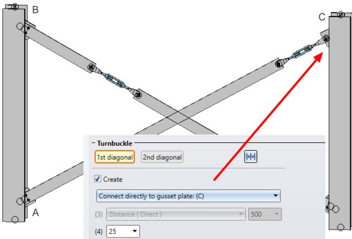
The turnbuckle of the first diagonal is connected directly to the gusset plate at point C, and the turnbuckle of the second diagonal is connected at both ends via a connecting plate.
