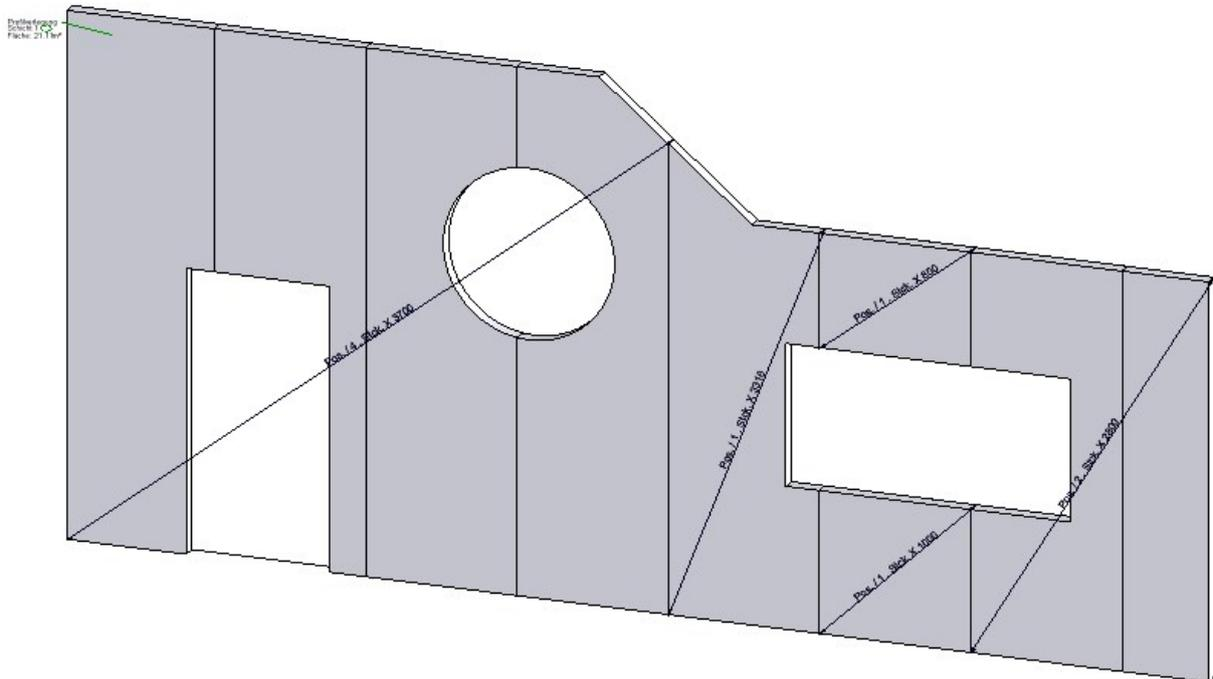
After selecting the function, the cut contour is displayed. Adjacent profiles of the same length are indicated by diagonal lines. The edits are also displayed.
