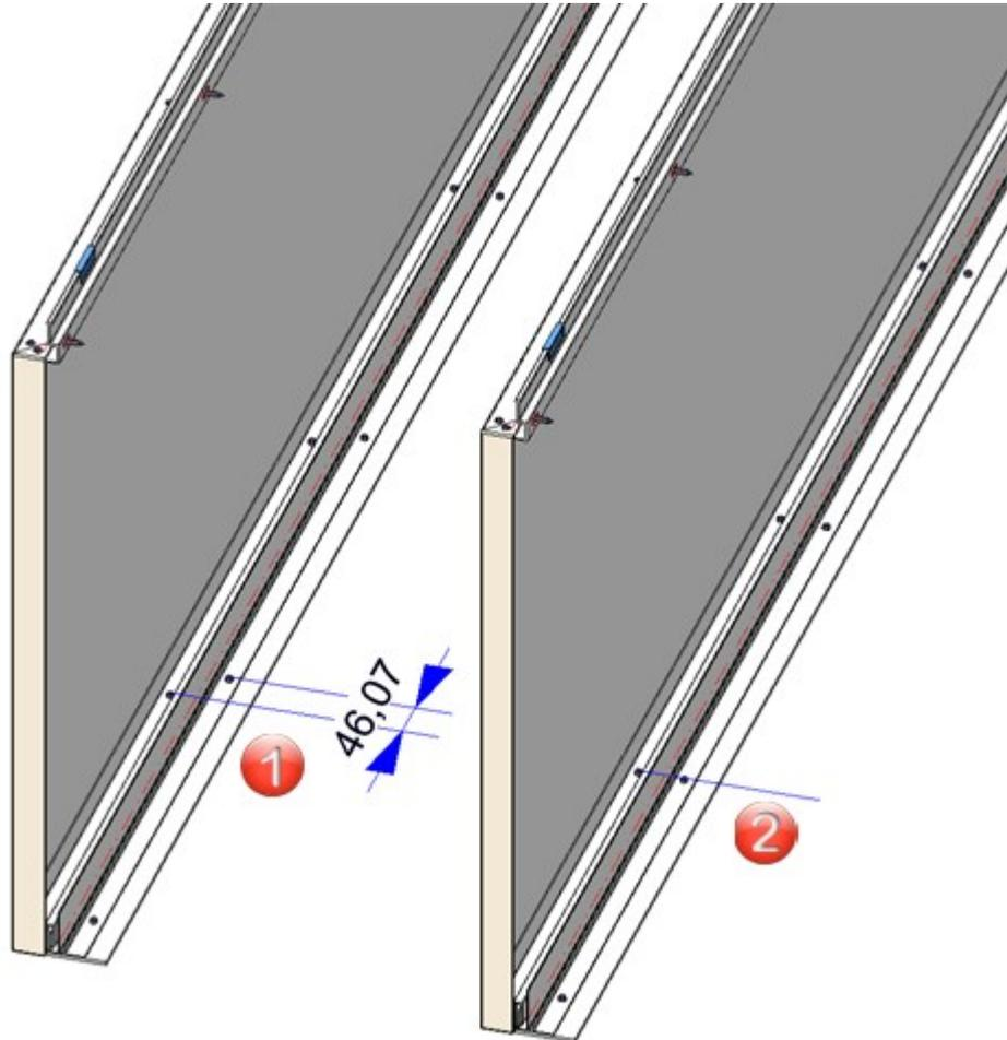
(1) Before HiCAD 2025 SP1, (2) Alignment of the rivets from SP1 in one line
