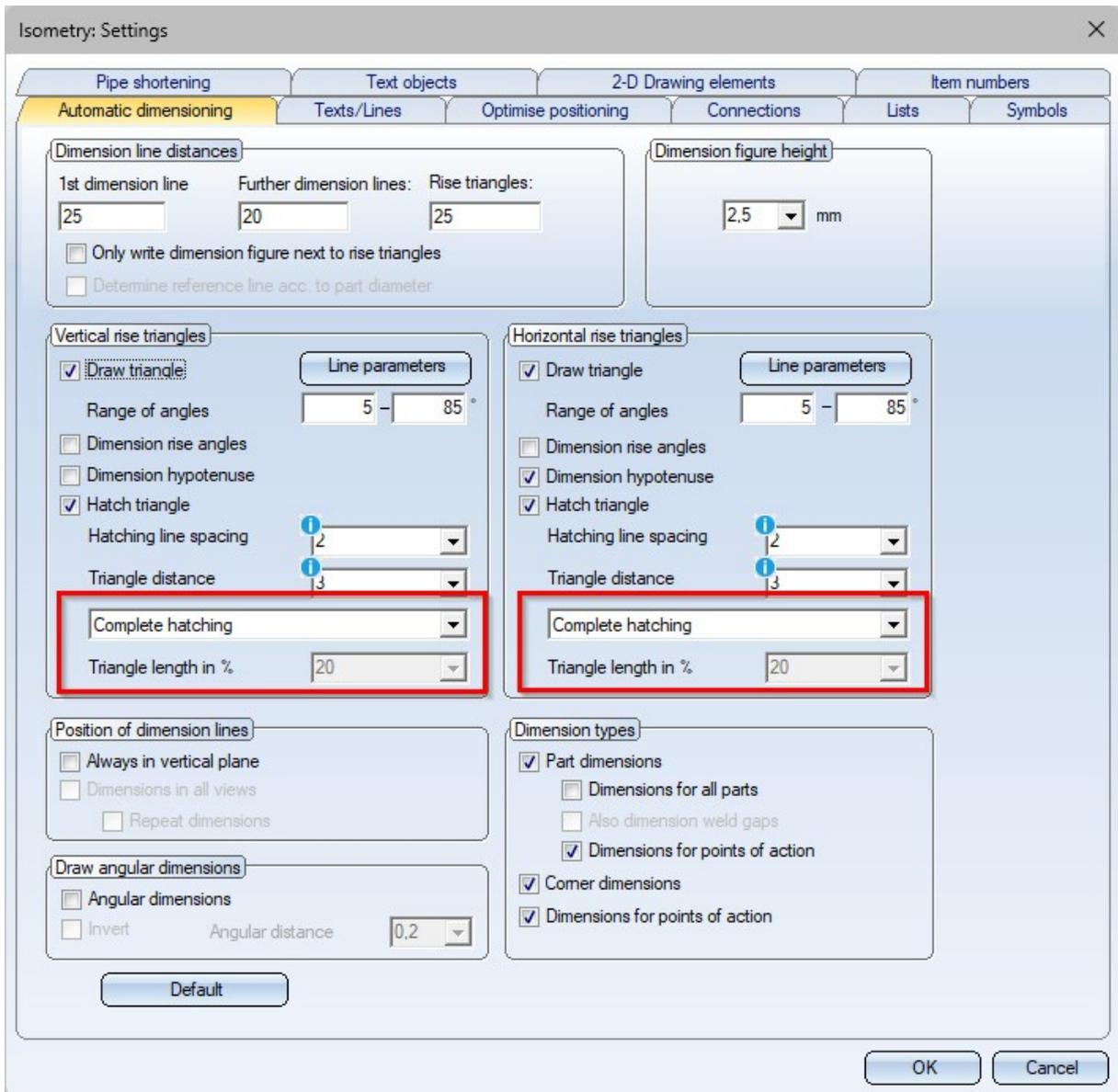
When a rise triangle is partially hatched, the hatched area is specified exclusively via the length of the base side of the rise triangle, and this is done proportionally in % to the length of the base side of the entire rise triangle. Before HiCAD 2025 SP1, the specification was in the length unit of the drawing.
