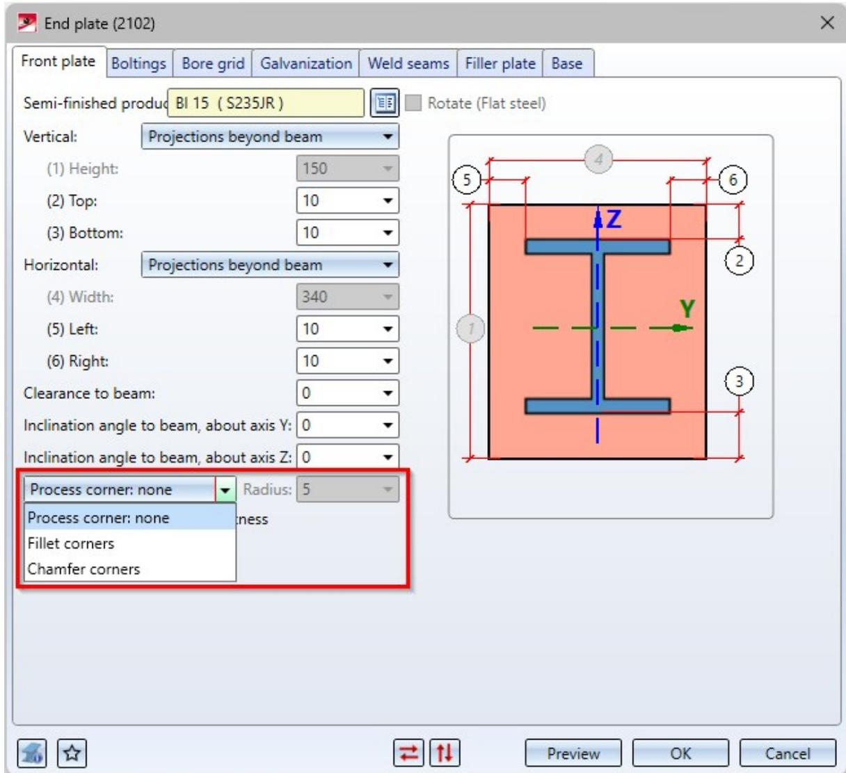
The chamfer angle is 45°, the length can be selected freely.
