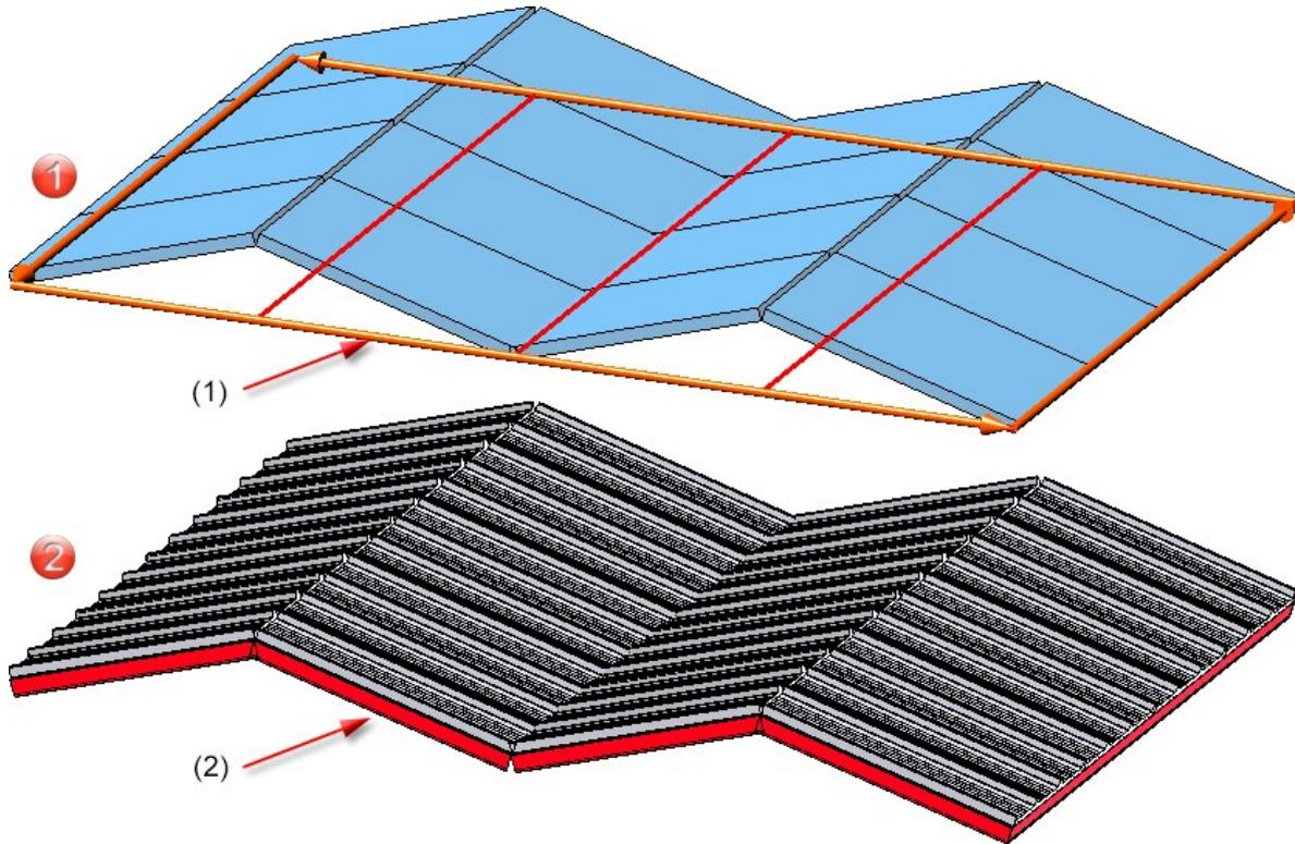
(1) Select the edges for the edge profiles using the sketch (orange arrows), (2) Edge profiles are adapted to the roof inclination
