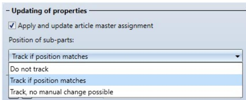
In the dialogue of the function **3-D Standard > New > Dependent part**
