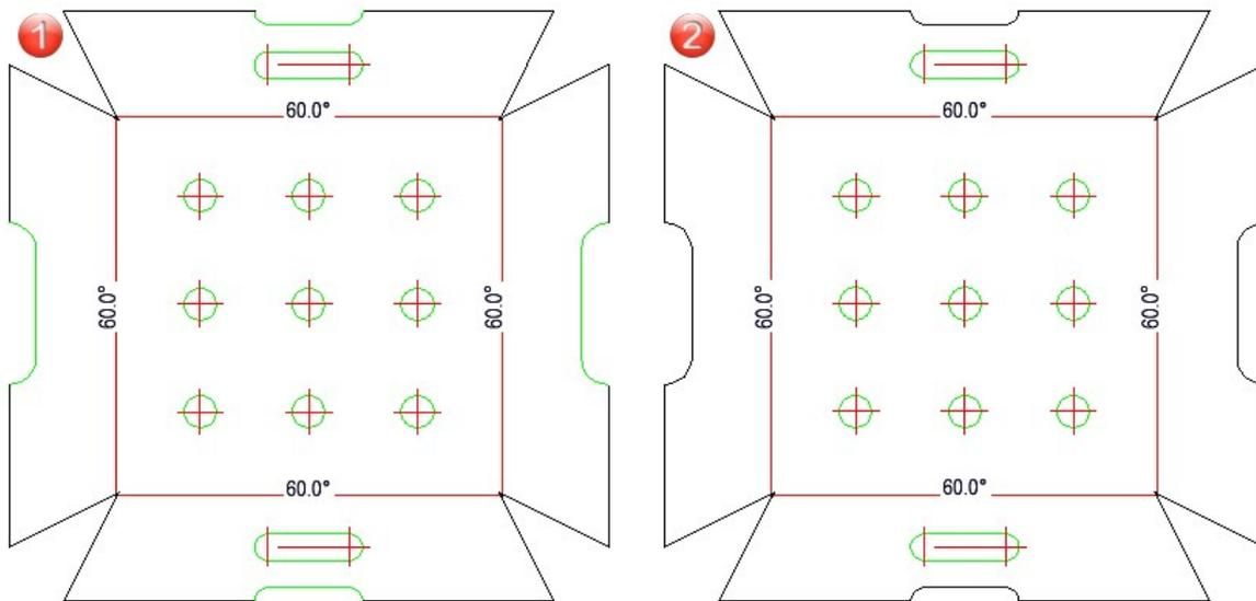
(1) Display of the outer contour before HiCAD 2025 SP1, (2) From SP1 onwards, standard parts on the contour are given the colour of the development edges.
