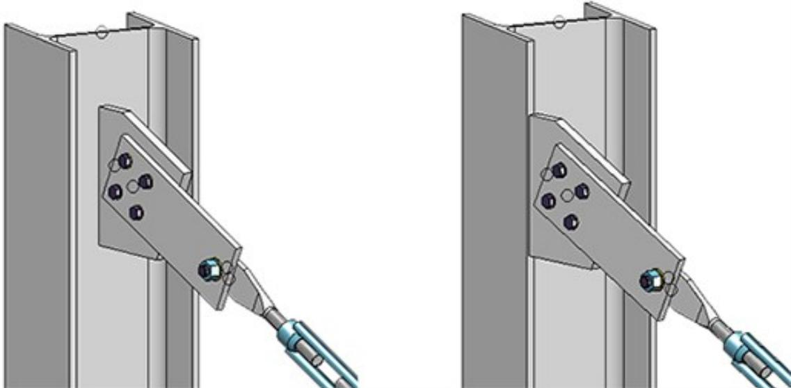
Left: Gusset plate mounted to web, right: Gusset plate mounted to front flange
