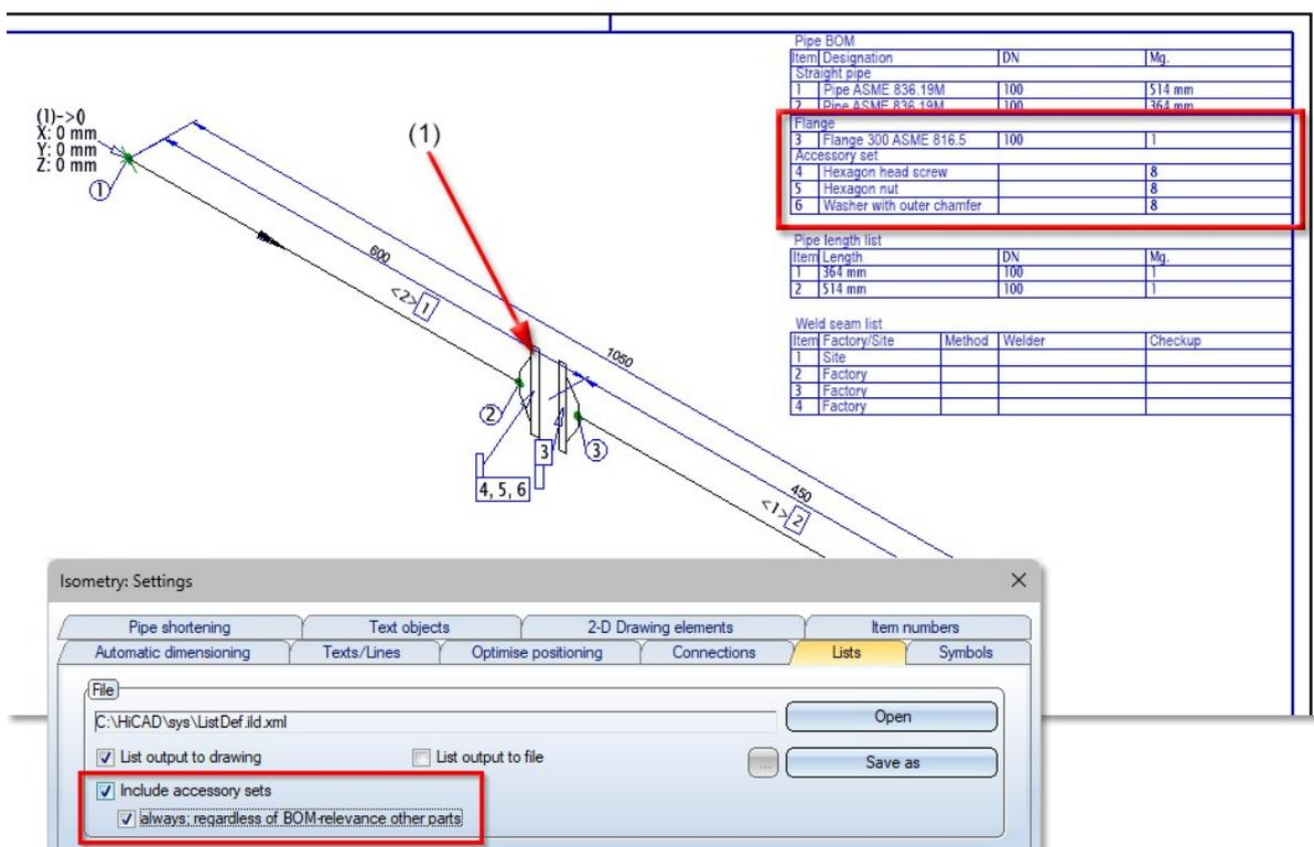
(1) The left flange is not BOM-relevant but has an accessory set. The right flange is BOM-relevant and has no accessory set.
