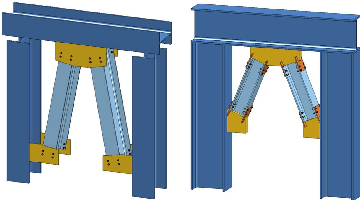
Left: Bolting of bracing members and gusset plates, Right: Bracing with slotted plates
