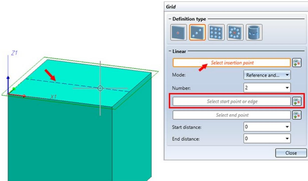
Preview line when selecting a point for a linear grid in the **Reference and Quantity** mode.
