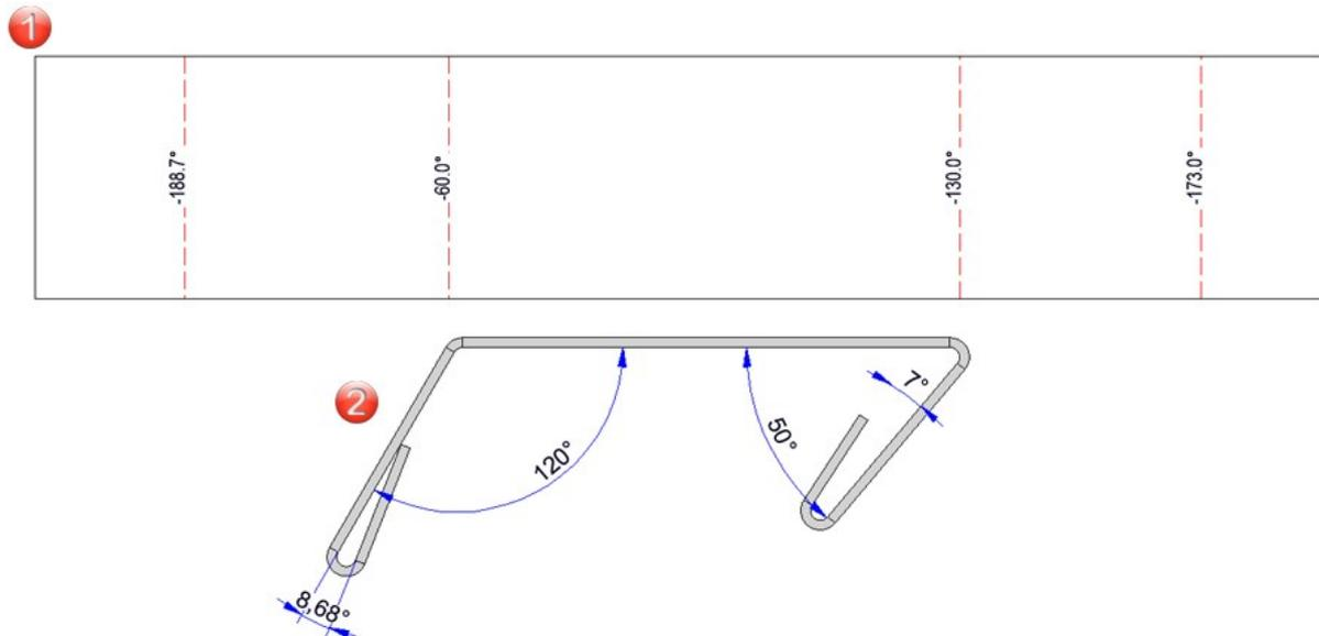
In this example, all angles with a negative sign are output when exporting with the setting **-3**. This seems wrong because the  $7^\circ$  angle (on the right in the picture) corresponds to a bend angle of  $173^\circ$  while the  $8.68^\circ$  angle (on the left) corresponds to a bend angle of  $188.7^\circ$ . However, this is the intended result when the setting **-3= neg. opening angle, also neg. angle for bend angle  $> 180^\circ$**  is used.
