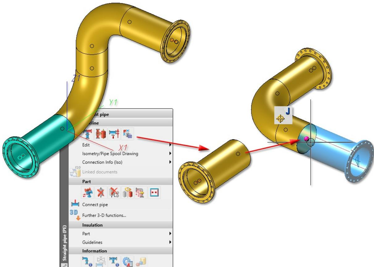
Pipe parts copied from Pipeline\_0001 (1) with guideline to Pipeline\_0002 (2) without guideline
