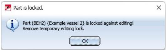
If a pipeline is locked, the following functions display a corresponding hint directly during the selection (some only if they are not called via context menu):
