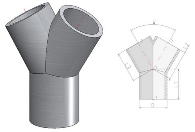
The geometry of these variants - in terms of outer diameter, wall thickness and the length of the "legs" - is based on the Y-piece YS.S from the company  $\text{HECO}^{\textcircled{R}}$ .
