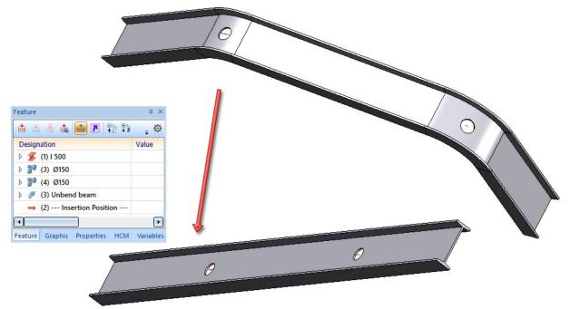
With HiCAD 2023 SP2 (V 2802) the geometric algorithm of the unbending calculation has changed. Therefore, there may be changes in the result. In particular, beams, which could also be unbent before, lie differently in space (see image). However, beams already unbent with a version before HiCAD 2023 SP2 will not be changed.
