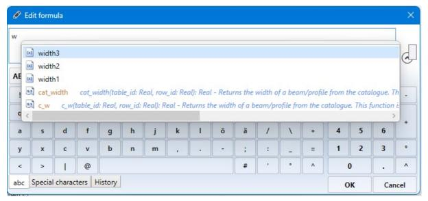
To display all formulas and variables, place the cursor in the input field and enter the key combination CTRL + Space bar.
