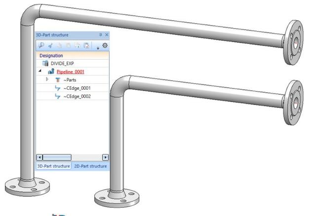
The **Divide pipeline** function has not supported the division of such a pipeline so far. As of HiCAD 2023 SP1, the system checks whether the pipeline to be divided consists of several connection components and indicates this - if so - at the cursor by a corresponding message.
