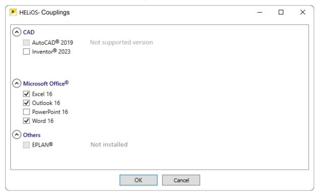
Activate the checkbox of the required software and confirm with **OK**. The interface will then be activated.
