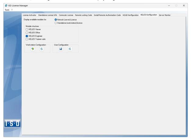
On the **HELiOS Configuration** of the **ISD License Manager** tool you have the option to save a workstation or user configuration for individual Clients.
