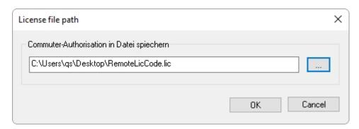
Here the Administrator enters the target path and the file name for the licenses to be swapped out. Make sure that a unique file name is used, for example, by including in the file name the host name of the remote computer and the expiry date.
