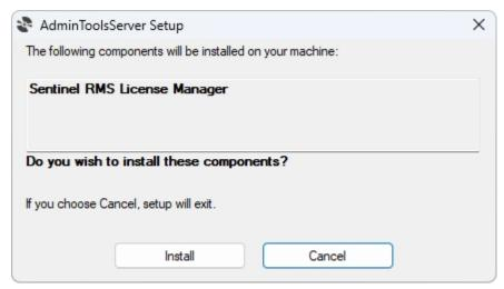
First, the system checks whether the Sentinel RMS License Manager is installed. If not, it is installed automatically.
