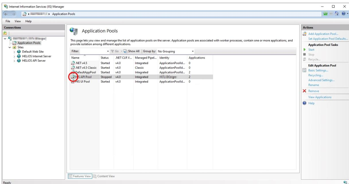
If the Application Pool has been terminated (as is the case in the screenshot above), this may be due to data or permissions that are stored for the user to run the Application Pool being incorrect.
