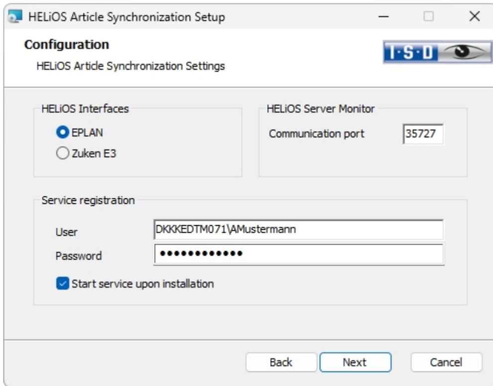
Choose the interfaced program and, in the **User** field, enter the User login for HELiOS, (or a user account) with access to HELiOS.
