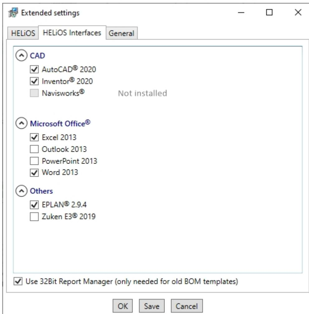
The availability of interfaces with HELiOS depends on the programs that are installed on your computer. You can only interface 64-Bit versions to HELiOS 64-Bit versions. An exception is the MS Office Interface, where you can link a 32-Bit Office to a 64-Bit HELiOS. Please note however that an additional, special ODBC connection will be required for old BOMs. In such cases, please contact the ISD Consulting team.
