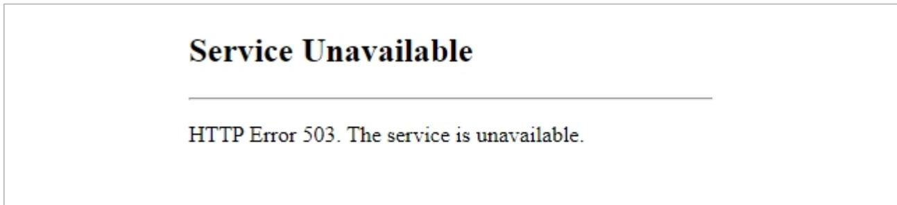
please check whether the Application Pool for the HELiOS API Server is running or if it has been terminated. This can be recognised by the icon or by the status display in the IIS Manager:
