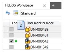
You can also insert parts into an active model drawing by moving them from the Workspace into the drawing with Drag & Drop.
