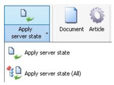
The **Apply server state** function checks whether the currently loaded document or the active document is identical with the current server state. If this is not the case- e.g. because the document has been saved by a different user in the meantime, or exists with a newer index, or because the master data of a linked article have changed or the article exists with a newer index - use this function to apply the current Server state to the document.
