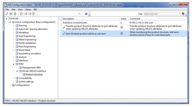
If a HiCAD model drawing (.SZA document) or an individual geometry (.KRA document) is saved in HELiOS while the option has been activated, it will be checked whether a semi-finished product needs to be saved as s structure sub-item of the corresponding part (=HELiOS article).
