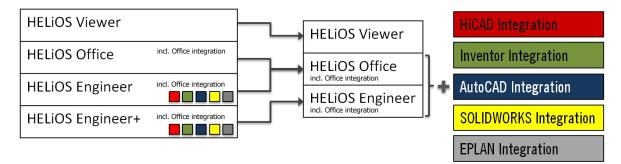
The Extension modules can be combined with HELiOS Office or HELiOS Engineer; in combination with HELiOS Office, only a purely document-based working will be possible. Without the integration modules, each HELiOS basic module offers at least the viewing functionalities for the corresponding CAD-/CAE application.
